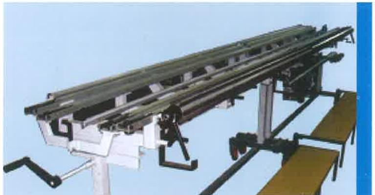
Separable Coupled Type For Twin Beam Looms
